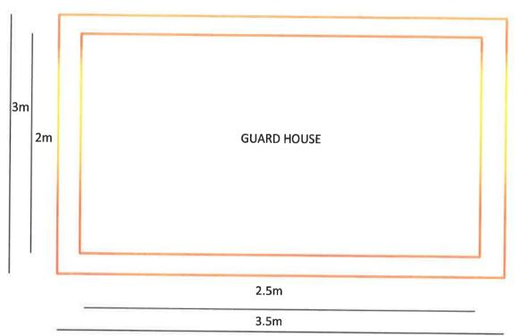
The guard house is 2,5x2m with a thickness of 0.1m (Slab), with a 0,5m apron on each side 3,5mx3mx0.1m = 1.05 m3
