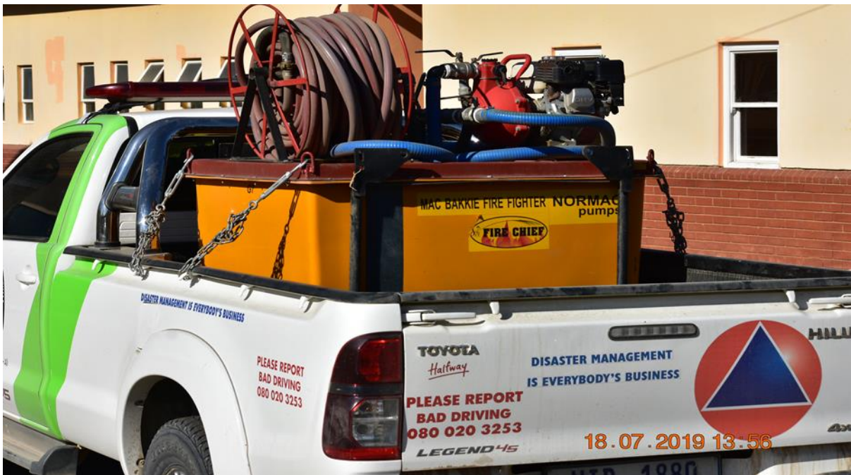
Figure 25- The skid unit procured by the municipality
